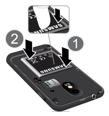
Replace the battery compartment cover, making sure all the tabs are secure and there are no gaps around the cover.
