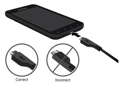
3. Plug the AC adapter into an electrical outlet. Fully charging a battery may take up to three hours.
