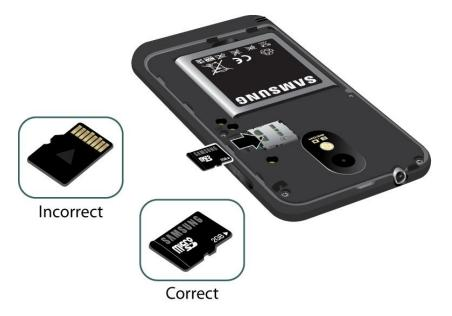
3. Firmly press the card into the slot and make sure that it catches with the push-click insertion.
