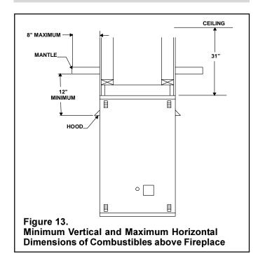
CAUTION: IF JOINTS BETWEEN THE FINISHED WALLS AND THE FIREPLACE SURROUND (TOP AND SIDES) ARE SEALED, A 300° F. MINIMUM SEALANT MATE-RIAL MUST BE USED. THESE JOINTS ARE NOT RE-QUIRED TO BE SEALED. ONLY NON-COMBUSTIBLE MATERIAL (USING 300° F. MINIMUM ADHESIVE, IF NEEDED) CAN BE APPLIED AS FACING TO THE FIRE-PLACE SURROUND. SEE THE DIAGRAM BELOW.
