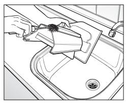
Clean the fabric conditioner channel with a brush and hot water. Liquid starch can cause the siphon to become clogged. Make sure that you clean the siphon and siphon tube particularly thoroughly after using liquid starch a few times.
