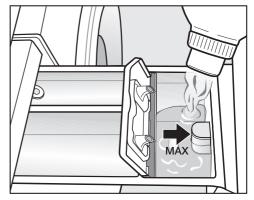
■ Add the fabric conditioner or liquid starch to the ⊗ compartment or insert the appropriate capsule. **Do not exceed the maximum level mark.**
