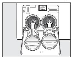
Replace the drain filters correctly (on the right and left) and tighten them securely.
