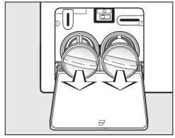
■ Remove the drain filters completely.
