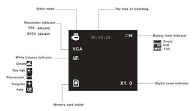
In Video mode, press the **OK/Menu** function button on the top right of the camera. The LCD will display 2 mode tabs – VIDEO and SETUP.
