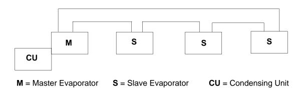
Each Beacon II board power is supplied by a transformer in the evaporator on which it is mounted. Do not run any 24 VAC wires between Beacon II boards on the evaporators.
