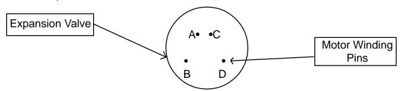
For valve sizes 29320003 and 29320004, the resistance measured between pin locations A and B or C and D should be approximately 336 Ohms when the valve is at 75°F.
