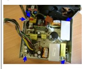
Figure 31:: Remove PSU FAN
