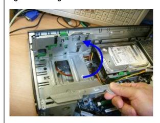
Figure 19: Rotate PSU to Vertical
