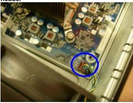
Figure 9: Remove fan and fan holder from chassis
