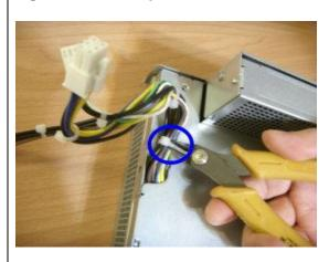
Figure 28: Remove PSU the top of case
