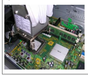
Figure 12: Press CPU chassis lock
