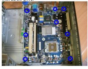
Figure 23: Remove PCA from Chassis
