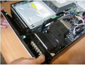
Figure 5: Remove all cable from cable clamp
