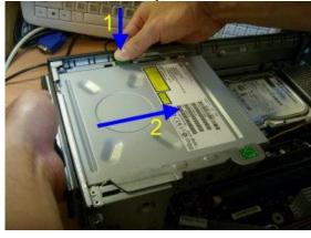
Figure 18: Rotage ODD cable to vertical
