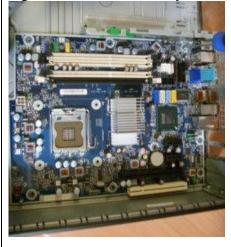
Figure 16: Remove all internal cable from PCA
