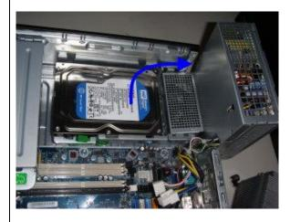
Figure 20: Release HDD Press HDD latch and push HDD toward Front side.
