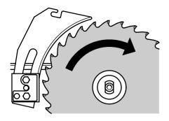
Danger! Use only suitable saw blades according to EN 847-1 (see"Technical Specifications" – when using unsuitable or damaged blades parts could be explosive-like hurled from it by centrifugal force.
