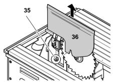
Hold saw spindle with 13 mm open 4. jaw wrench and loosen arbor bolt (37) with Allen key (L.H. thread!).
