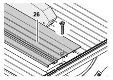
3. Loosen screws (27) of the riving knife bracket.
