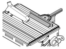
The auxiliary fence extrusion can be taken off and reversed after loosening the two screws (23), (25):
