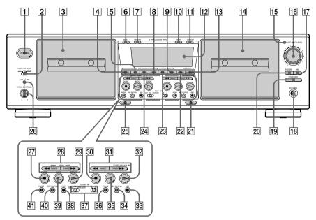
A + B REC 22 (15)ARL 17 (12) AUTO indicator [15] (10, 12) CHECK 24 (9) Deck A 3 (7, 20) DECK A 23 (11) Deck B 14 (10, 20) DECK B 9 (11) DIRECTION MODE 2 (7, 10) Display 12 DISPLAY 8 (9) DOLBY NR 37 (7, 10) FADER 20 (13) HIGH/NORMAL 13 (14) MEMORY (on deck A) [7] (8) MEMORY (on deck B) 11 (8) PHONES jack 18 PITCH CONTROL 26 (7) POWER **1** (7, 10)
