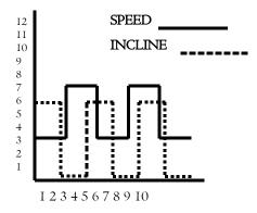
\*The Cross Training Program is designed to control the walking belt speed and elevation inversely in alternating segments.
