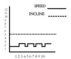
The **Cardio Program** is designed to vary the treadmill Speed, while maintaining a constant Elevation.
