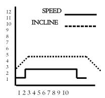
The Warm Up Program is designed to gradually increase the treadmill Speed and Elevation in the first segment (warm up) and gradually decrease the treadmill Speed and Elevation in the last segment (cool down). This is also known as a Plateau program.
