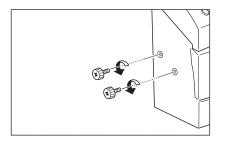
Attach the handset cradle to the fax using the screws provided with the handset. Do not use the screws originally attached to the fax.
