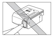
Do not touch the print head area on the BJ cartridge. Ink may leak out and cause stains.
