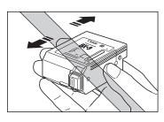
Never shake the BJ cartridge, especially after removing the protective tape from the print head.
