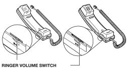
Adjust the volume of the ringer. Use a pen or other pointed object to adjust the switch to HIGH, LOW, or OFF.
