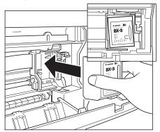
The yellow post (BJ cartridge guide) should be visible through the slot. The BJ cartridge tilts slightly to the left in the loaded position.
