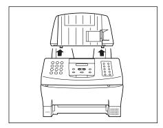
2 Fan a small stack of up to 100 sheets (up to 10 mm thick). Tap the edge of the stack on a flat surface to even the stack.
