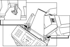
Make sure the stack of paper does not exceed the paper limit mark on the right side of the paper tray.
