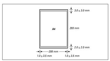
The margin on either side of the sheet and the margin on the top and bottom are not picked up by the scanner.
