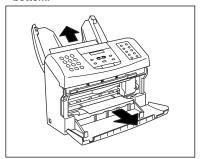
6 Load the paper (see Loading the paper, p. 7), then replace the paper tray cover, and press [Stop].
