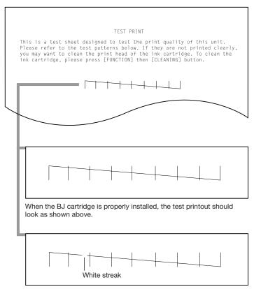
If the printout has white streaks as shown above, try cleaning the print head. See Cleaning the BJ cartridge print head, p. 104. If the problem persists after cleaning, try reinstalling the BJ cartridge.
