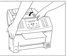
While holding the operation panel open, pull the sheet out from the top or bottom.
