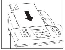
The fax automatically feeds the pages one by one from the bottom.
