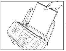
4 Holding the paper stack, squeeze and slide the paper guide until it touches the left edge of the stack of paper.
