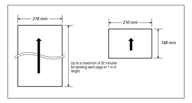
The actual scanned image size for the fax is shown below.
