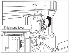
Make sure the paper thickness lever is set to the paper position (left position).
