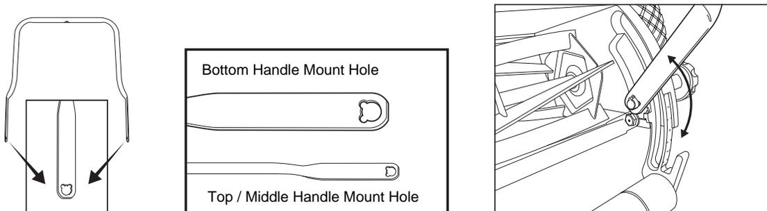
3. Continue assembly of the middle and top sections of the handle using the handle bolts and wing nuts.
