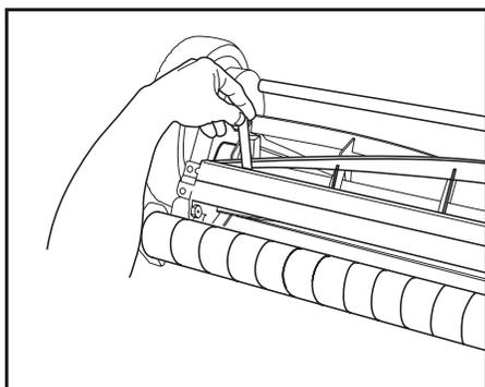
5. The blades may also be tested by inserting a piece of paper vertically into the blades while turning them by hand.
