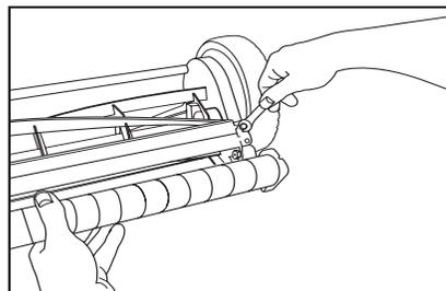
3. Make the same adjustment at the other end of the cutting bar.
