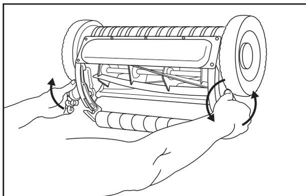
2. Set the height, using the scale on the back of the roller arms, to the same setting on both sides and re-tighten the black knobs. The mower is now ready to mow at the desired height setting.
