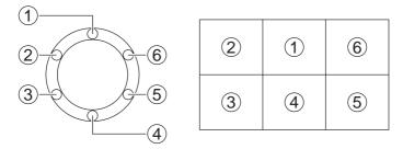
Example 1. When the camera detects a person in area (1) on the display.
