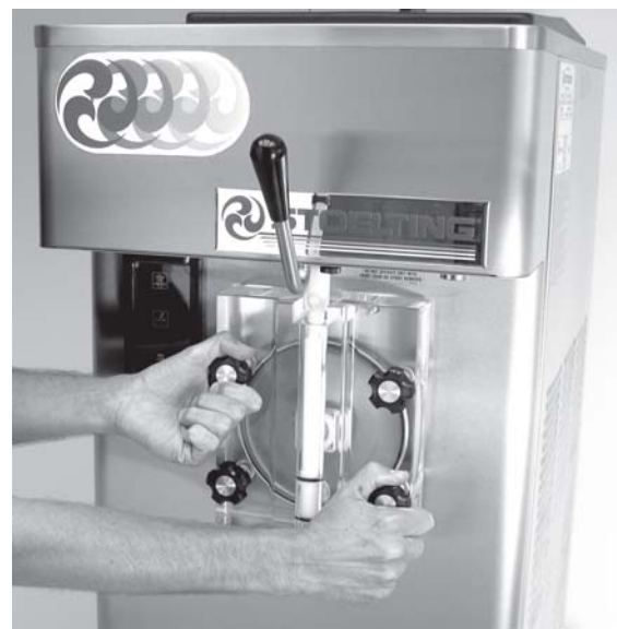
Figure 14. Removing Front Door
