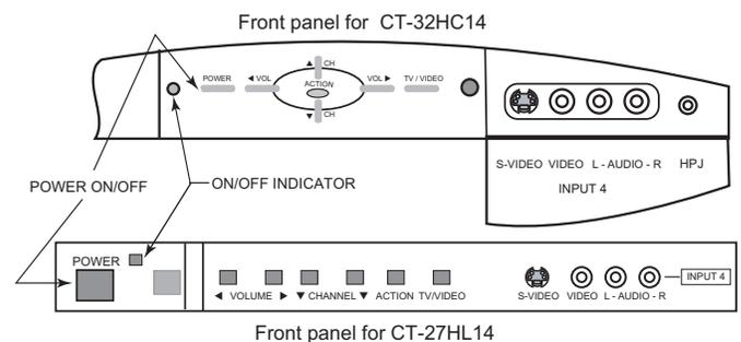
A second VCR, Camcorder, a video disc player, video game equipment or DSS equipment can also be connected to the video inputs. See the optional equipment manual for details.
