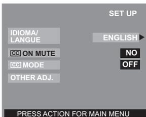
☐ **CC MODE** - This television contains a built-in decoder that displays **CC** (Closed Captioned) text across the screen (white or colored letters on black background). It allows the viewer to read the dialogue of a television program or other information. The program viewed must include Closed Captioning for the feature to work. Activate the onscreen Closed Caption feature by selecting one of the following modes.
